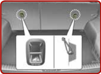
Securing with "Tether Anchorage" system [3]
