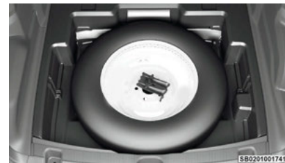
Damaged Tire Stowage
