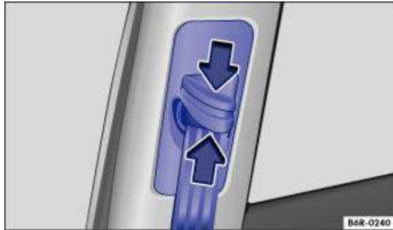
Fig. 58 Next to the front seats: belt height adjuster
