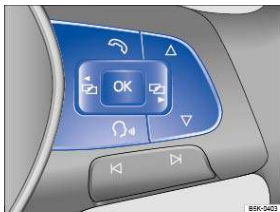
Fig. 16 Right-hand side of the multifunction steering wheel: controls for using the menus and information displays in the instrument cluster
