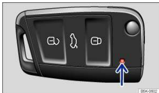
Fig. 23 Indicator lamp in the vehicle key
