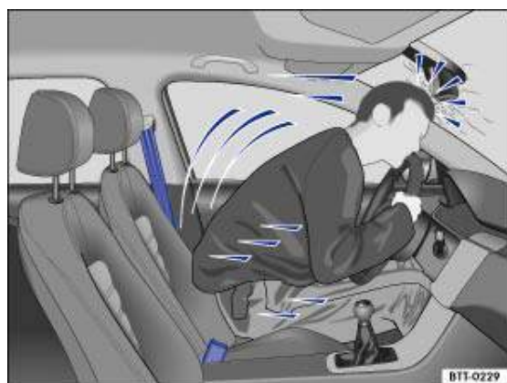
Fig. 51 An unbelted driver is thrown forwards
