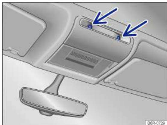
Fig. 30 In the roof console: sensors for the interior monitoring system (arrows)
